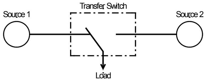
Figure 3-11: Open transition switch - connected to source 1
