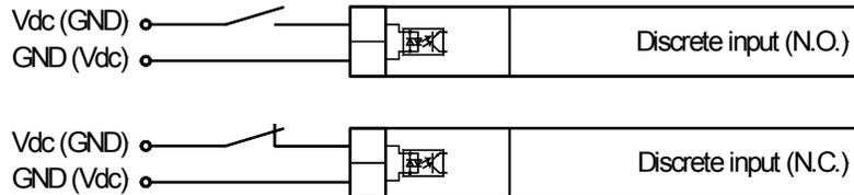
Figure 3-27: Discrete inputs - control inputs - operation logic
