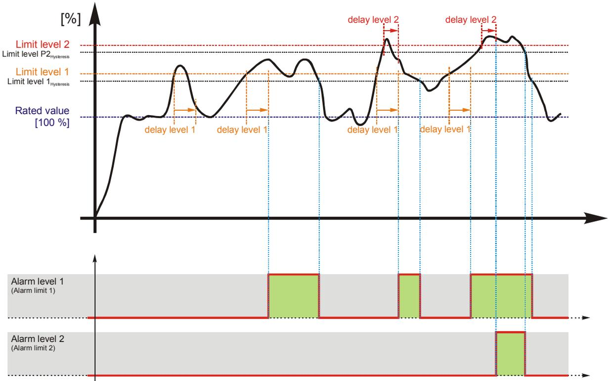
Figure 3-25: Monitoring - battery overvoltage
