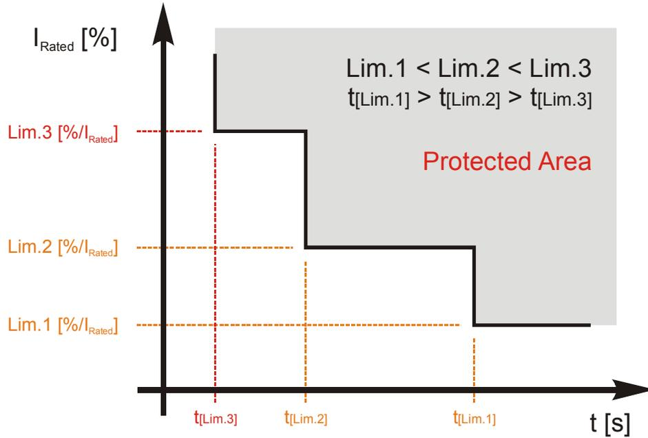
Figure 3-23: Monitoring - load time-overcurrent
