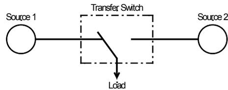
Figure 3-16: Closed transition switch - connected to source 1
