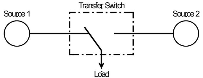
Figure 3-13: Delayed transition switch - connected to source 1
