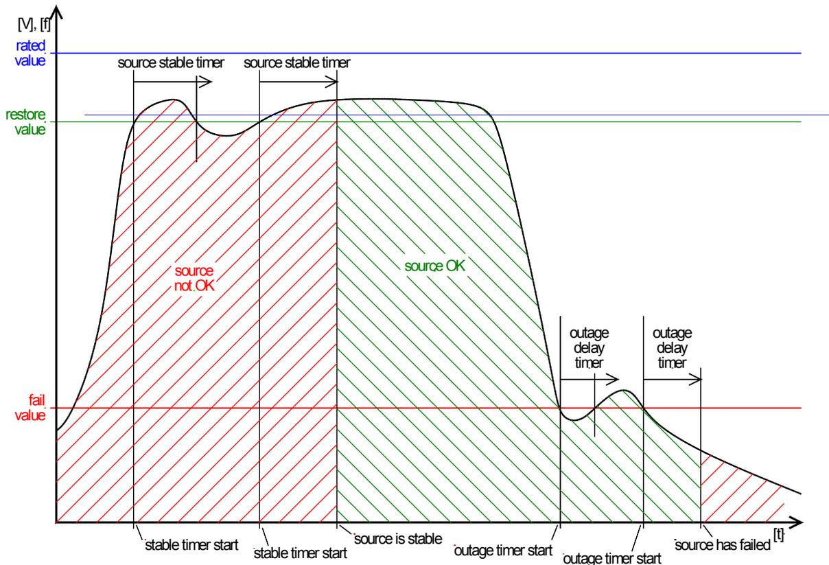
Figure 3-2: Source stable and outage timers
