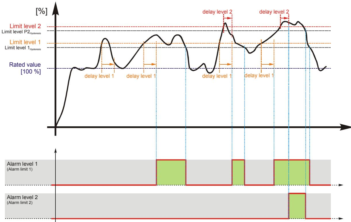
Figure 3-24: Monitoring - overload
