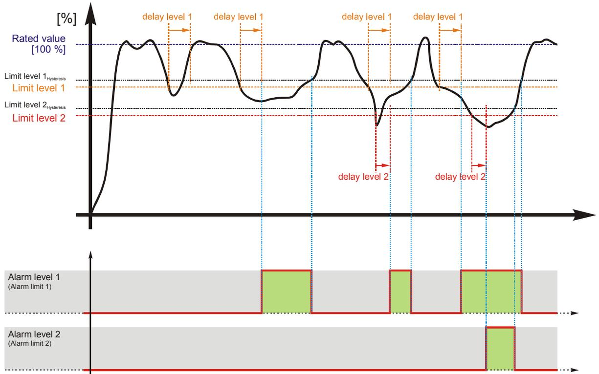
Figure 3-26: Monitoring - battery undervoltage
