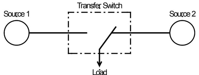
Figure 3-15: Delayed transition switch - connected to source 2
