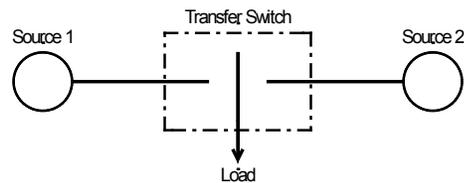
Figure 3-17: Closed transition switch - neutral position
