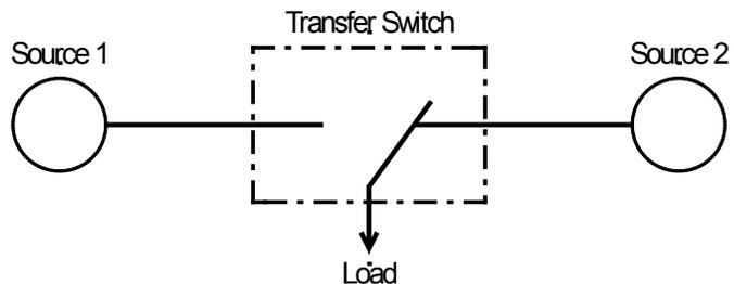
Figure 3-12: Open transition switch - connected to source 2
