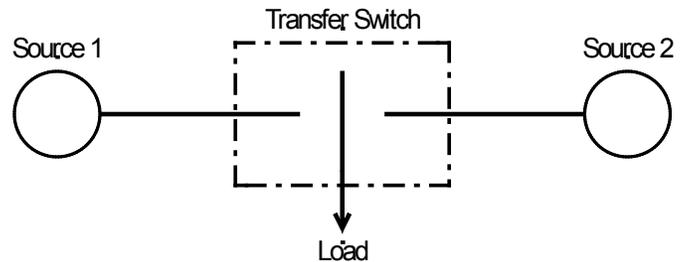
Figure 3-14: Delayed transition switch - neutral position
