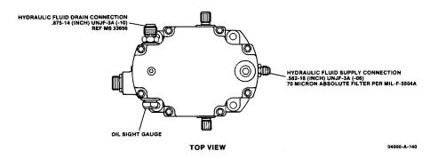
Figure 2. Oil Line Connections for TG-13E and TG-17E Which Require a Customer-Supplied Hydraulic Pressure Source, but do not Require a Drive
