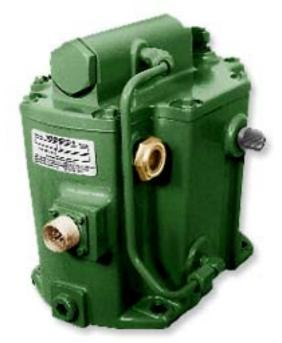
driving such loads as alternators, dc generators pumps, compressors, fans or paper-making machines. The actuators provide the "muscle" for a Woodward 2301, 2500, 501 (with a digital remote final driver), or similar integrating electronic control system. The actuators provide a mechanical output position in proportion to a dc control signal.
