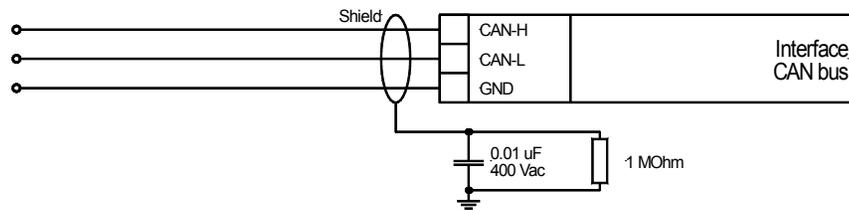
Figure 3-11: Shielded wiring
