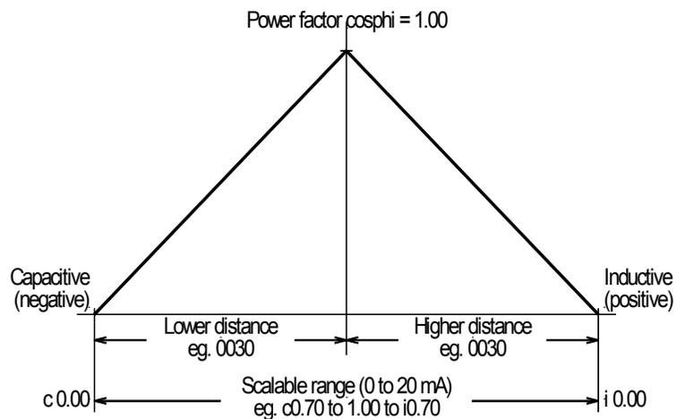
Figure 7-7: Analog outputs - power factor scaling
