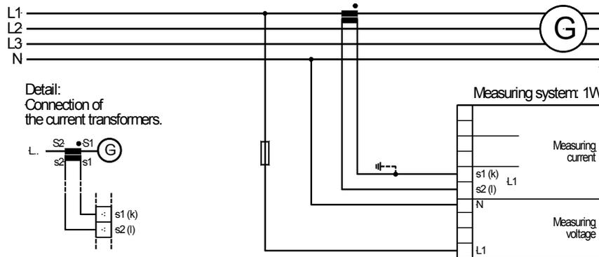
Figure 7-1: 1W measuring system
