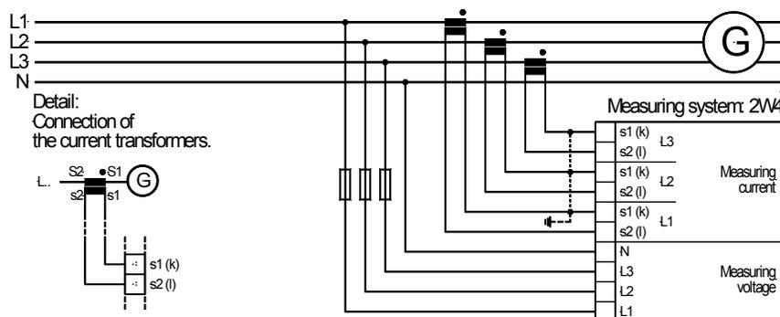
Figure 7-5: 2W4 measuring system
