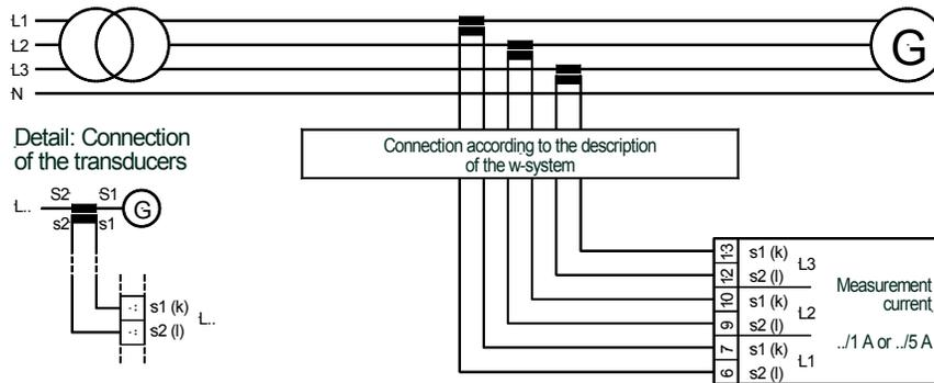
Figure 3-6: Measuring inputs - current 100/400 V versions
