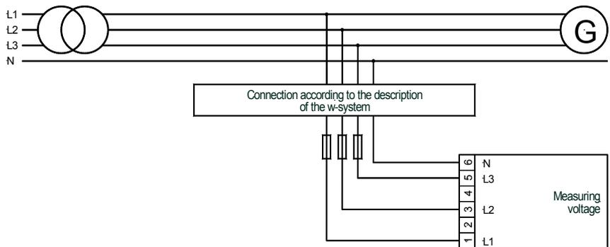
Figure 3-5: Measuring inputs - voltage, 690 V version
