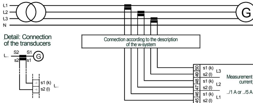
Figure 3-7: Measuring inputs - current, 690 V version
