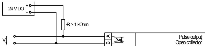
Figure 3-9: Impulse output
