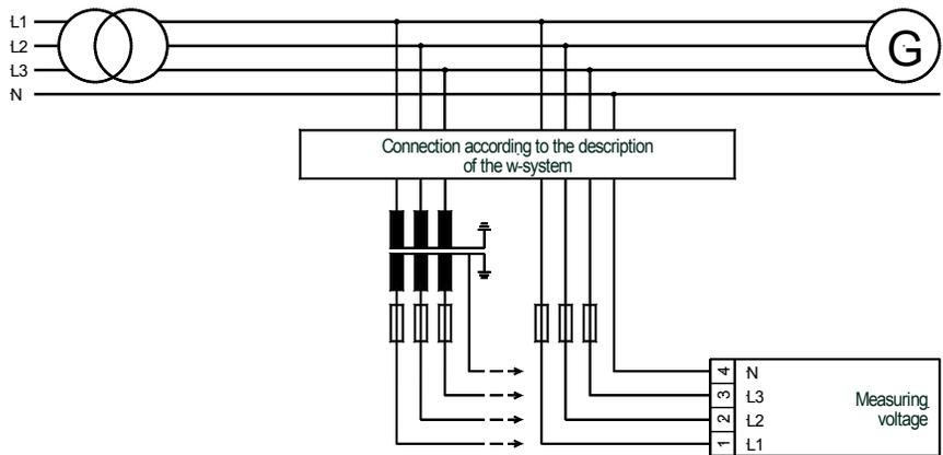
Figure 3-4: Measuring inputs - voltage 100/400 V versions
